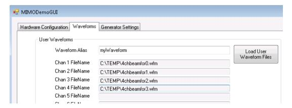
The Rx Waveforms tab lets you load individual waveforms, or load a set of waveforms from a CSV configuration file. It also allows you to override the waveform playback settings of sample rate, RMS value, and scale factor.
