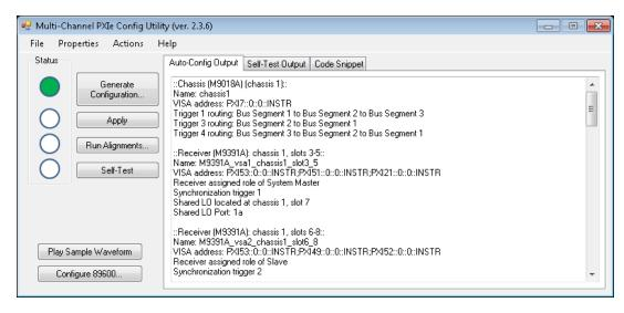
Clicking on the 'Apply' button will connect to the M9018A chassis and M9300A reference to make any changes necessary to operate multi-channel VSGs and VSAs. Changes are not made to the VSGs or VSAs at this stage (multi-channel VSG and VSA
