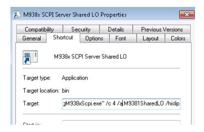
To set up the M9381A SCPI server, you first need to create IVI config store entries that share a common name, but end in -#, where # is the channel # of the VSG, beginning with 1. For example, a 2-channel VSG might have IVI config store entries of M9381SharedLO-1 and M9381SharedLO-2. The first channel should be the master channel for purposes of synchronization. Note that the Multi-channel Config Utility can be used to automatically create these IVI config store entries.
