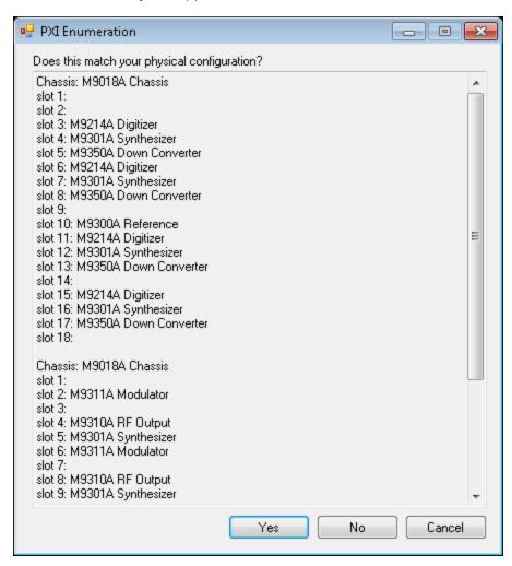
Occasionally, some modules can be missing from this list. This usually means that the Keysight IO Libraries has not finished enumerating all devices. If this occurs, close the application and try again in a few minutes.
