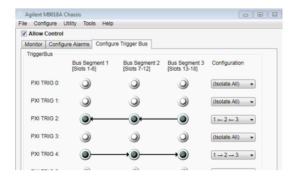
The synchronization scheme requires one PXI trigger per VSG or VSA channel. One group trigger must be allocated from a "master" M9311A or M9214A module in each chassis to all of the other M9311A or M9214A modules. Additionally, each "slave" M9311A or M9214A module must use a unique synchronization trigger routed to the "master".
