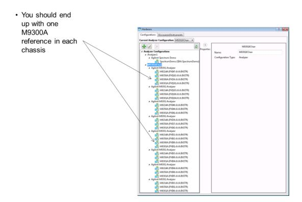
The master channel in each chassis must have a reference module selected in addition, and the other channels must not have one selected. By convention, the master channel is the first (topmost) in the list of configurations for the first chassis. The master channel for the second chassis (if present), can be at any position, but should be first among the modules for the second chassis.
