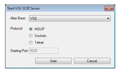
You can select an alias base name from the drop down. Only VSG base names with the required number of channels for the current configuration will be displayed. You can also select which protocol you would like to use: HiSLIP, Sockets, and Telnet. For the Sockets and Telnet options, you may also specify which starting port number you would like to use. Clicking the 'Start' button will launch the VSG SCPI server.
