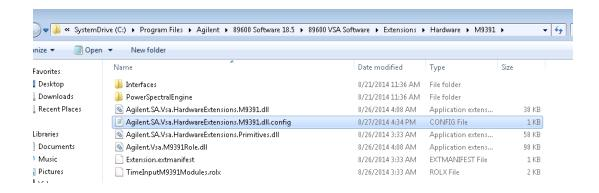
Prior to 89600 release 19.0, if multi-chassis configurations are set up, a configuration file must be created which maps the analyzer channels to a set of chassis slots. This will enable the 89600 M9391 driver to correctly set up the multi-chassis synchronization. After the configuration file is placed in the hardware extension directory, for example: C:\Program Files\Keysight\89600 Software 18.7\89600 VSA
