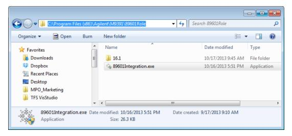
89600 VSA software will support up to 8 channels of M9391A VSA. When the M9391A VSA driver software is installed, it also installs the 89600 drivers (role) if 89600 VSA is already installed. If 89600 VSA software is installed after M9391A software, the 89600 drivers may be missing. In this case, you can run the 89600 integration script, which is available from the M9391A applications in the start menu.
