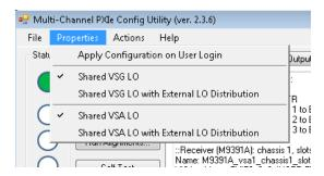
By default (no option selected) the system will be configured to run with independent synthesizers (Independent LO). This means that each VSG or VSA will need to have its own synthesizer to provide a LO signal. This allows for the VSGs and VSAs to set independent center frequencies to perform tests for applications like carrier aggregation. Independent LO configured systems are not phase locked.
