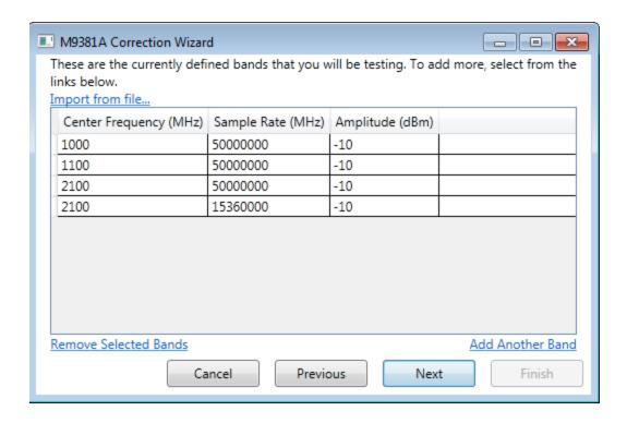
The M9381A Correction Utility measures the timing and phase delta between up to 8 channels of M9381A using a combiner with the output fed into a single channel VSA. Currently an M9391A analyzer is supported via the IVI driver, or an analyzer connected to the 89600 VSA software. The software connects to the M9381A VSGs via a running SCPI server, over hislip connections. After hardware connections are
