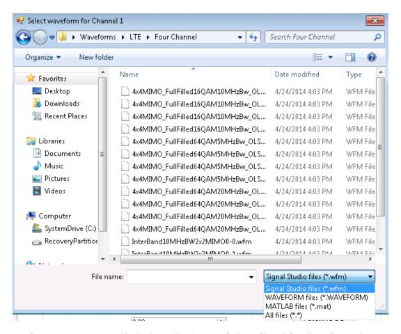
Waveform types supported include MATLAB .mat IQ data, Signal Studio .wfm, and MXG-compatible .WAVEFORM files. Consult the SCPI documentation for the M9381A's :MEM:COPY command for other supported file types. The SCPI documentation can be located on a typical installation via the Start menu, or in the filesystem here:
