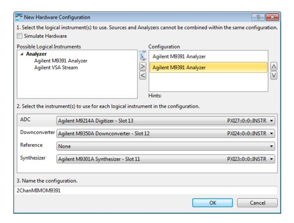
Configuration Dialog. M9391A must have a digitizer, downconverter, and synthesizer module selected.
