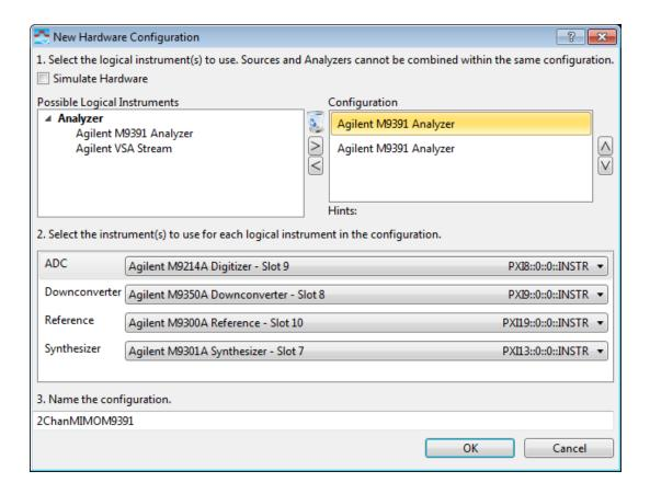
To set up the 89600 hardware configuration you will add up to 4 Keysight M9391 Analyzers to the configuration using the "New Hardware Configuration" dialog. Each of these must be populated with modules from the discovered hardware. 89600 automatically discovers any modules that could be used to make up an M9391A VSA. If you start 89600 too soon, prior to complete PXI enumeration by the operating system, you can always re-run the hardware discovery from the Hardware
